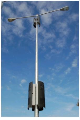
CommScope has devised a new two-piece concealment solution that will make deployment of metro cells on street poles much easier. (Photo: Business Wire)
