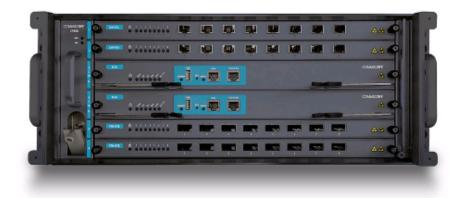
The C9516 EPON OLT, is the cable industry's first temperature-hardened, DPoE enabled, 10-Gigabit EPON OLT, specially manufactured to withstand extended temperature range environments while delivering enhanced functionality. (Photo: Business Wire)
