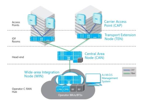
The CPRI interface solution will link Nokia's AirScale baseband unit to CommScope's Era™ C-RAN antenna system to dramatically reduce the time, space and power required. (Graphic: Business Wire)
